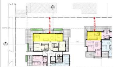
Figure 11: Extract of Plan 5 showing the setbacks to the boundaries with 18 and 18A Crabbes Avenue, Area of contravention highlighted yellow. (Source: Hyecorp/AmglenCity Plan)
