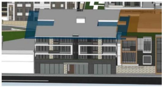
Figure 4: Extract of Height Plane Diagram. Development above the blue height plane representing the extent of the contravention (Source: Hyecorp)
